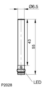
**Inductive Sensors** BES 516-371-G-S 49-C D6.5 x 55 normally-open Sn=2mm shielded
